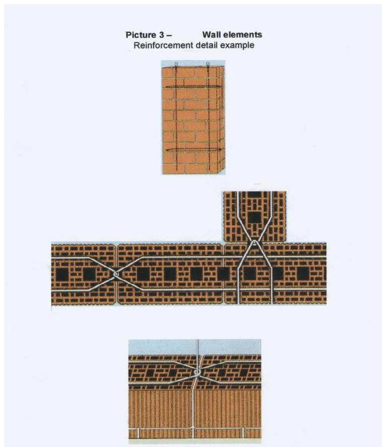
The walls and the ceiling is connected together with the rebars, making building resistant to the horizontal seismic loads and the vertical loads, a sample detail can be seen in picture 4.
